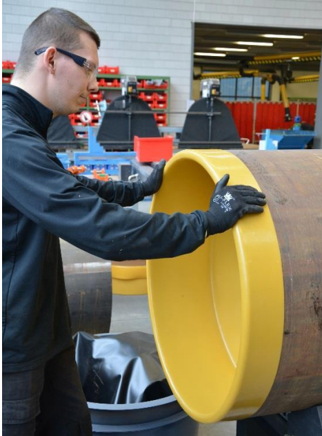
Step 5. Gently push around the circumference of the Recessed Cap
