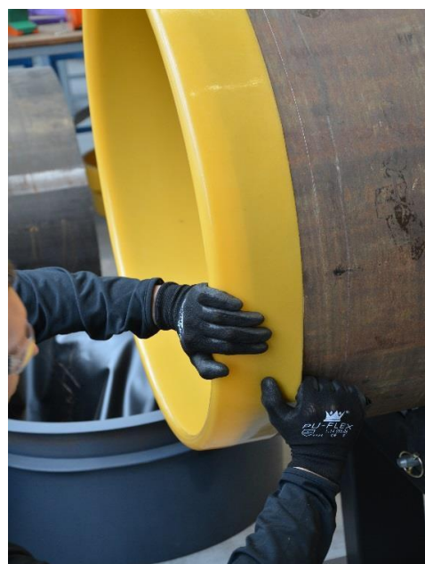
Step 4. Use the Application and removal Tool to apply the Recessed Cap completely into the pipe
