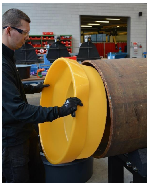
Step 4. Remove the Recessed Cap from the pipe
