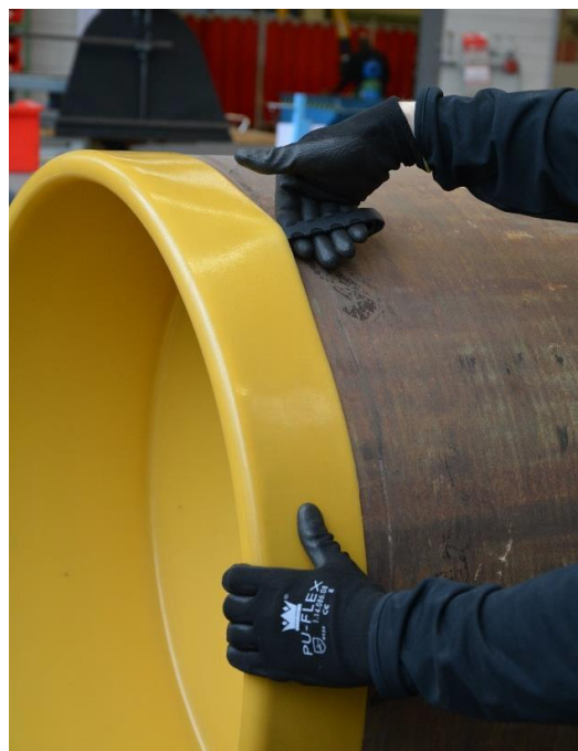
Step 2. Use the Application and Removal Tool to make the removal process more easy
