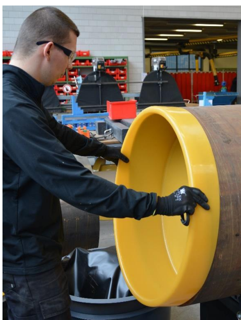
Step 3. Take the Recessed Cap out of the pipe end
