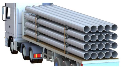
Figure 21. Place remaining layers
