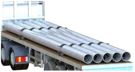
Figure 17. Place Anti-skid on the bottom layer (Truck only)
