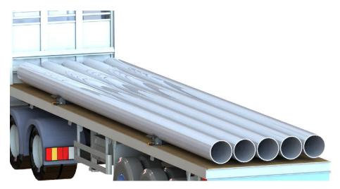
Figure 16. Place pipes on the bottom blocks
