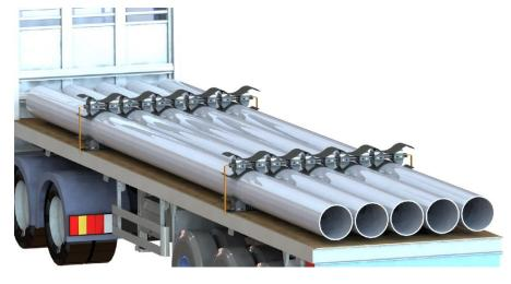
Figure 20. Place Anti-skid on the mid-section (Truck only)
