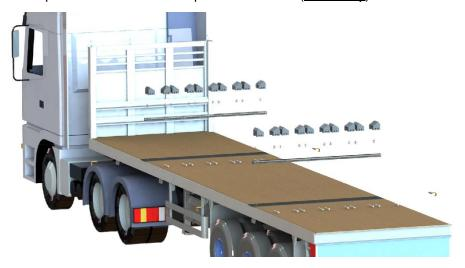
Figure 11. Start set-up with Anti-skid in place (trucks only)
