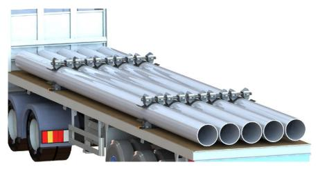
Figure 18. Place the mid-section with blocks on top of the bottom layer
