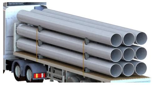
Figure 21. Place remaining layers
