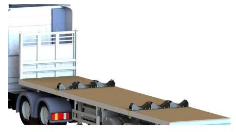
Figure 15. Place Anti-Skid on top of the blocks (truck only)
