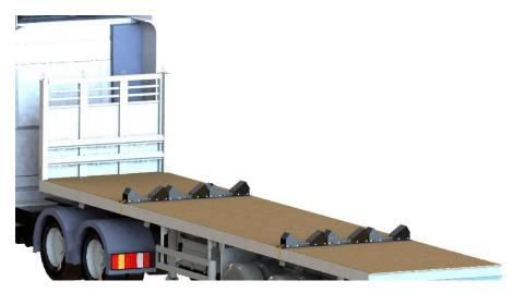
Figure 14. Lock the blocks with a pin and place profile-to-trailer connectors
