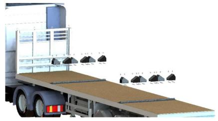
Figure 12. Fasten profile to trailer
