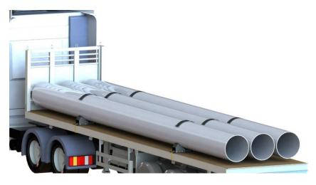
Figure 17. Place Anti-skid on the bottom layer (Trucks only)
